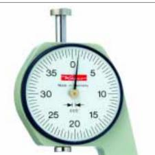
Pocket Dial Thickness Gauge JZ 15.005"Reading.400"Range.400"Range per revolution
