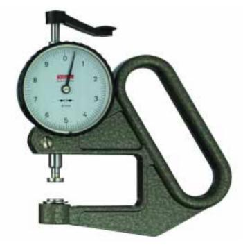
Model **K 50 with lifting device** has the same technical specification as model K 50 with pressure lever. At rest the feelers are closed. This style has the advantage that the contact pressure of 0,5 N is applied independently of the user. The **Spare Dial Gauge for K 50 with lifting device** will be supplied without lifting device unless requested on the order.
