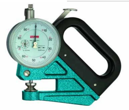
The predecessor model F 1000/30 of the new Foil Dial Thickness Gauge F 1101/30 is still available. One revolution of the pointer equals 0,2 mm corresponding to 200 graduations. Its measuring pressure is approximately 2 N. If required it can be supplied with a higher measuring force of 4,5 N or with a lower measuring force of 1,2 N.
