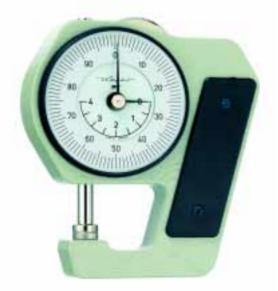
At rest the feelers on models KZ 15 and KZ 15/2 are open. Pushing the button on top of the instrument brings them together.
