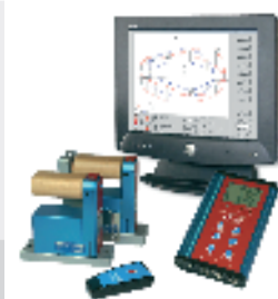
Two BlueLEVEL BASIC with BlueMETER BASIC and Laptop with measuring software
